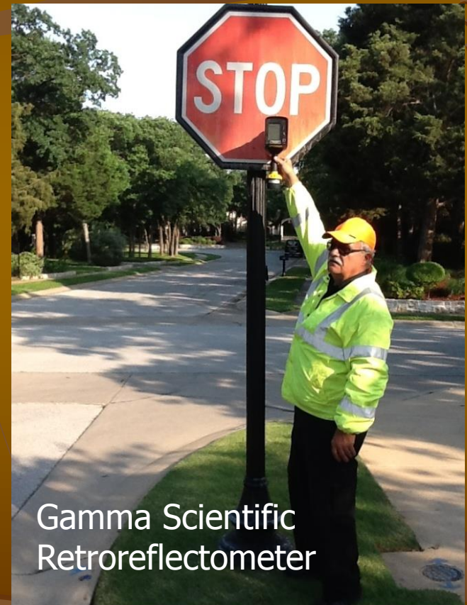
Faded & Damaged Street Sign Retroreflective Sheeting Assessment Evaluation
