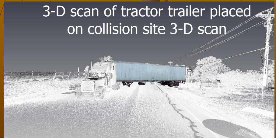
3-D scanning of crashed truck tractor (Stopper & Associates Mobile Forensic Unit in background)
